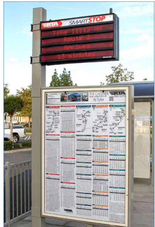
FIGURE 22: KIOSK WITH ATIS MODULE
